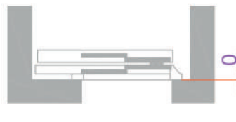
Installation of the shaft door directly in the shaft
